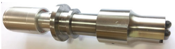
Fig. 6.7 Ultrasonic assembly for FSW integration
