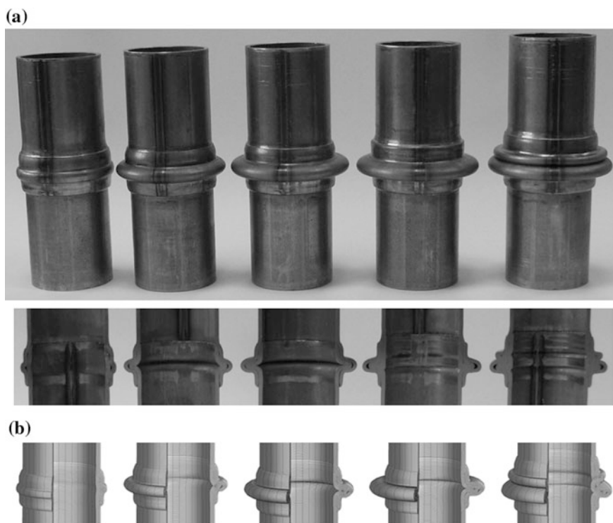
Fig. 7.8 Modes of deformation as a function of the slenderness ratio l_{\text{gap}}/r_0 when attempting to connect tubes by their ends with the new proposed technology. a Experimental results with cross-section details of the joints and b associated finite element predictions
