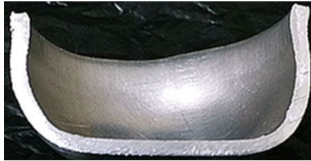
Fig. 6.17 Thickness variations along the wall of a successfully drawn cup
